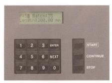
Wire program screen (shown above) displays program number, batch quantity, and wire length in inches, millimeters or centimeters. Other screens are used to program optional wire marker, select one of six languages, and display set-up, diagnostic and other data.
