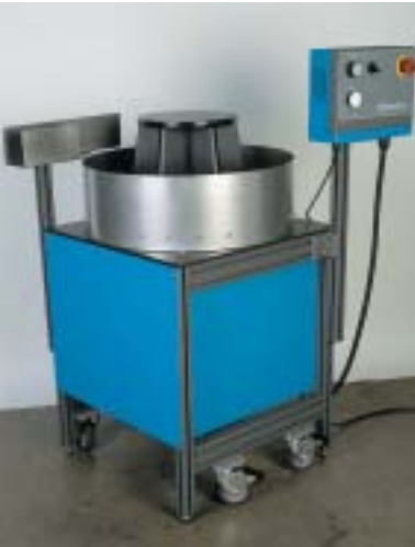
Model 16800 collects long lengths of wire or cable as it is processed.
